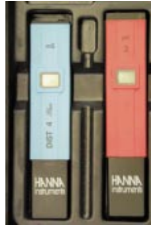
Figure 68: Simple digital pH and Ec meters
