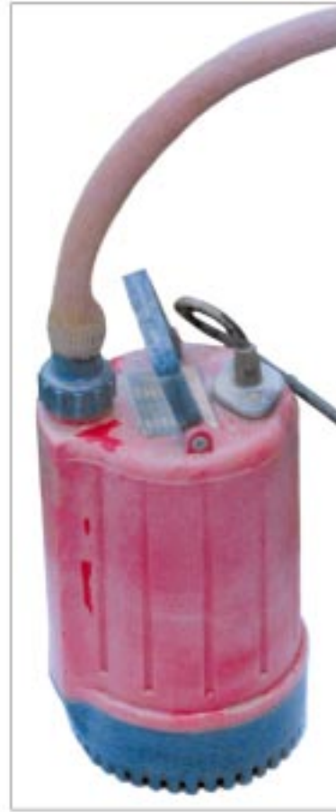
Figure 66: A submersible water pump
